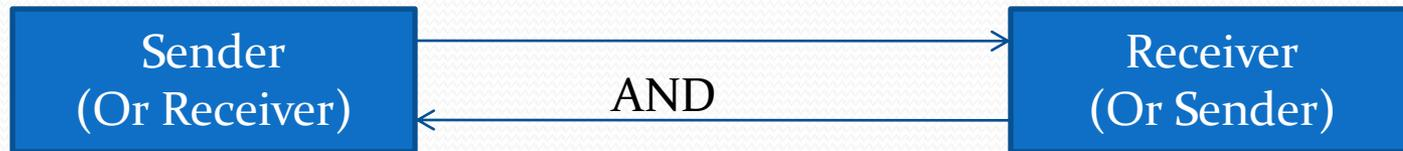
This mode requires four wires that allows data to flow in both directions simultaneously. Modern computer and internet are most popular examples of this mode. It improves efficiency because it eliminates the direction switching delay of a half duplex system
