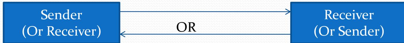
A Half Duplex communication system can transmit data in both direction., but in only one direction at a time. Hence, it can alternately send and receives data. It requires two wires. it is most suitable for voice communication using telephones in which open person can speak at a time.
